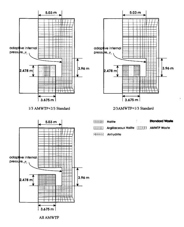
Figure 7. Computational mesh and boundary conditions for combined and supercompacted waste configurations.
