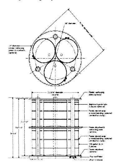
Figure 2. Six 100-gallon drum payload assembly (DOE 2000, Figure 2.1-7).
