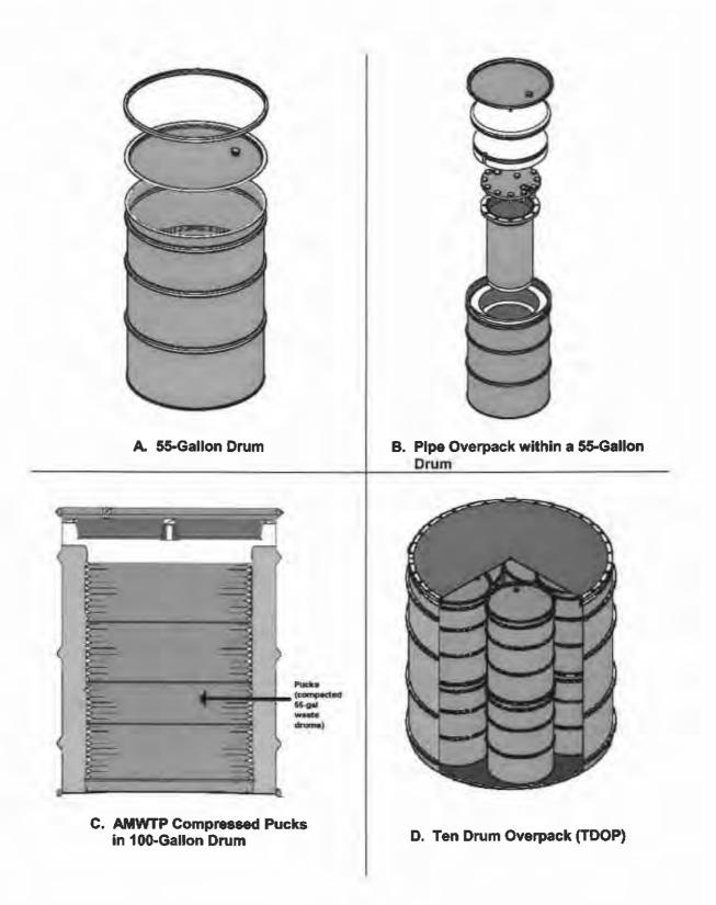
Figure 5. Illustrations of structural differences in waste containers.
