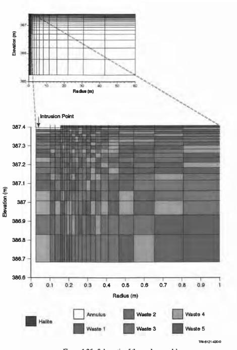
Figure 4-26. Schematic of the random model.
